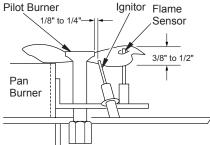
Figure 19 - Correct Pilot Flame Pattern -Electronic Assembly
